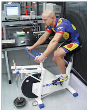
Ergometer modified to record WANt using BIOPAC
